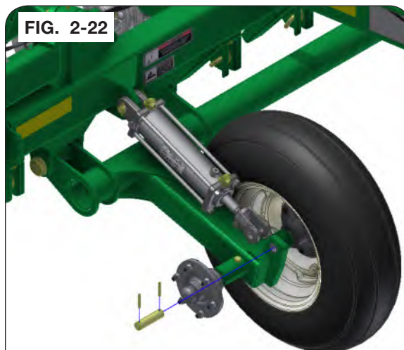
1" Dia. x 4" Pin (85631) & 1/4" Dia. x 1 7/8" Spiral Pins (91144-165)
